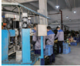
Machinery workshop Auto pin-drilling machine, auto threading machine, bending machine, drilling machines, all helps to reduce the labour cost and get higher efficiency.
